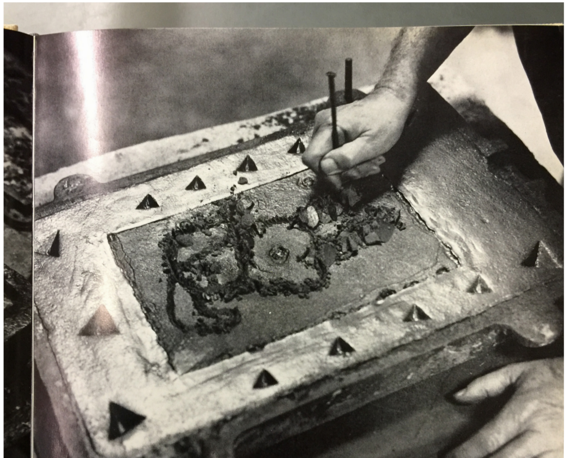
Bas-Relief, Bronze, 1969 by Juan Miró where also the downsprue becomes part of the sculpture, below: photograph shows him scratching directly into the sand mold
